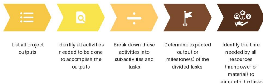
Figure 3: Development steps of a Work Breakdown Structure
